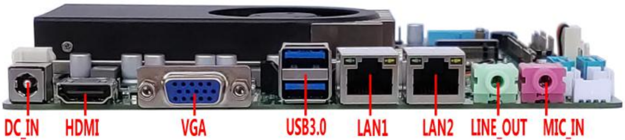
VGA + dual lan port picture ↓
